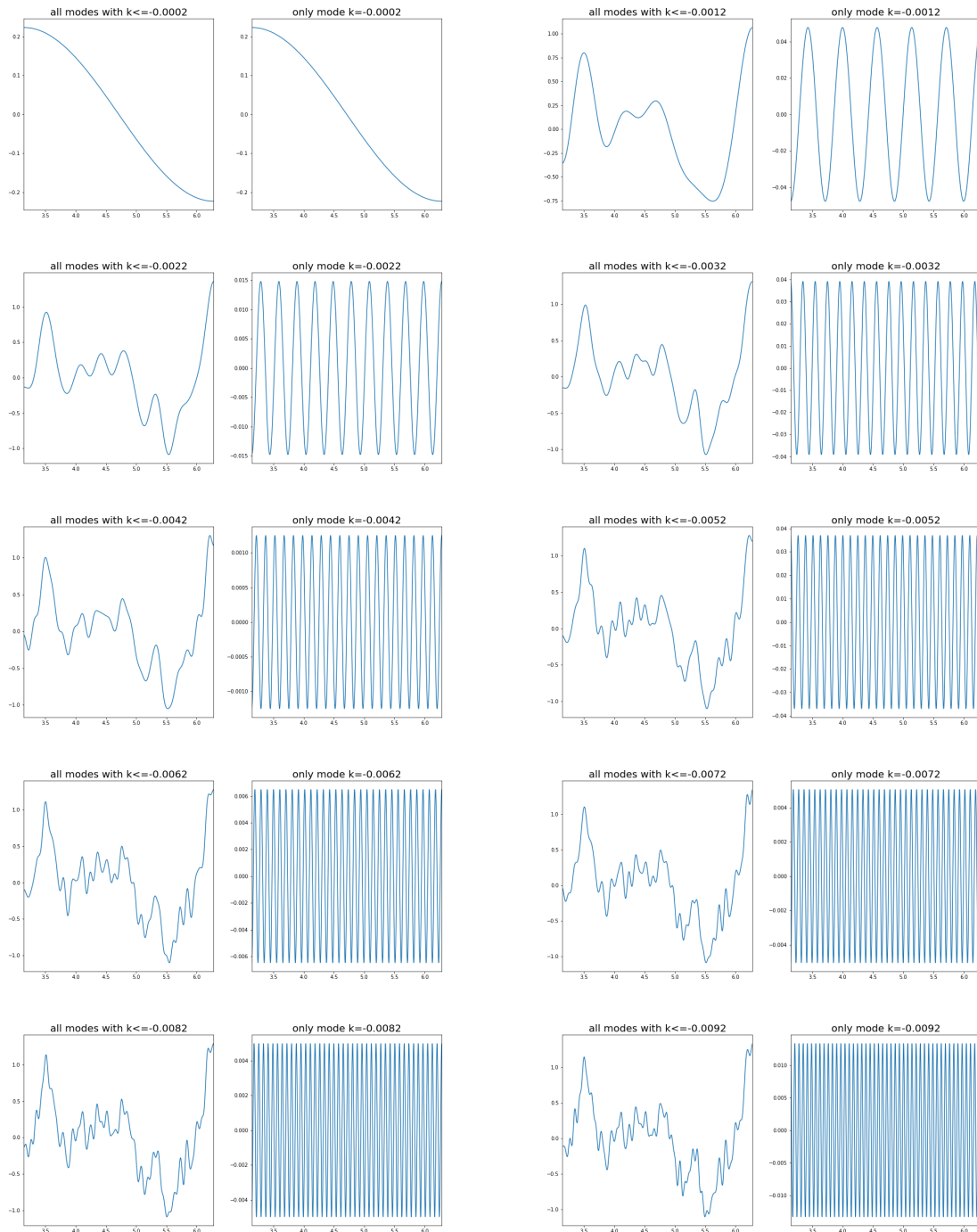
Figure 3: Impact of the individual modes on a 1D Gaussian random field following a power spectrum in k^{-2} . Each one of the 10 plots shows the contribution of a specific mode (the right part) and the sum of all the contributions of the modes lower and equal to this mode.
