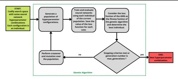
FIG. 1. Diagram of neural network hyperparameter tuning with a genetic algorithm.
