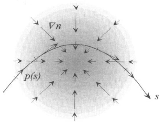
**Figure 2.** The space gradient of the refractive index changes the ray tangent as it passes through an inhomogeneous region.
