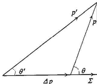
**Figure 3.** Ibn Sahl's diagram for refraction. A ray incident on a surface with normal  $\Sigma$  has direction  $p$ ; the increment  $\Delta p$  is parallel to  $\Sigma$ . The refracted ray has direction  $p'$  such that the ratio of vector lengths  $|p|$  and  $|p'|$  is the ratio of the refractive indices,  $n/n'$ . The common right side of the two triangles is the conserved quantity.
