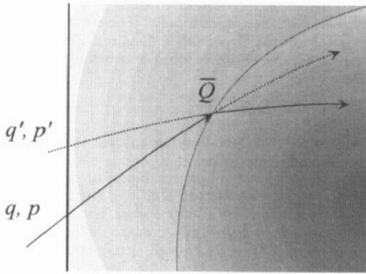
**Figure 4.** Refraction is a factorizable transformation between the initial points of the incident  $(q, p)$  and refracted rays  $(q', p')$  lying on a reference plane.
