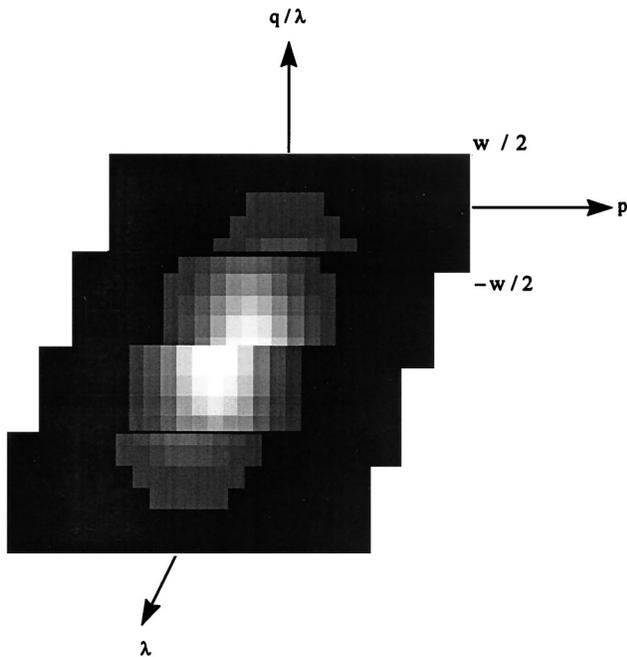
Fig. 6. Multiple copies of the original Wigner function after the plane of the slit. In this way each copy bears a different portion of the signal and is capable of passing the information through the spatial neck of the finite-width aperture.
