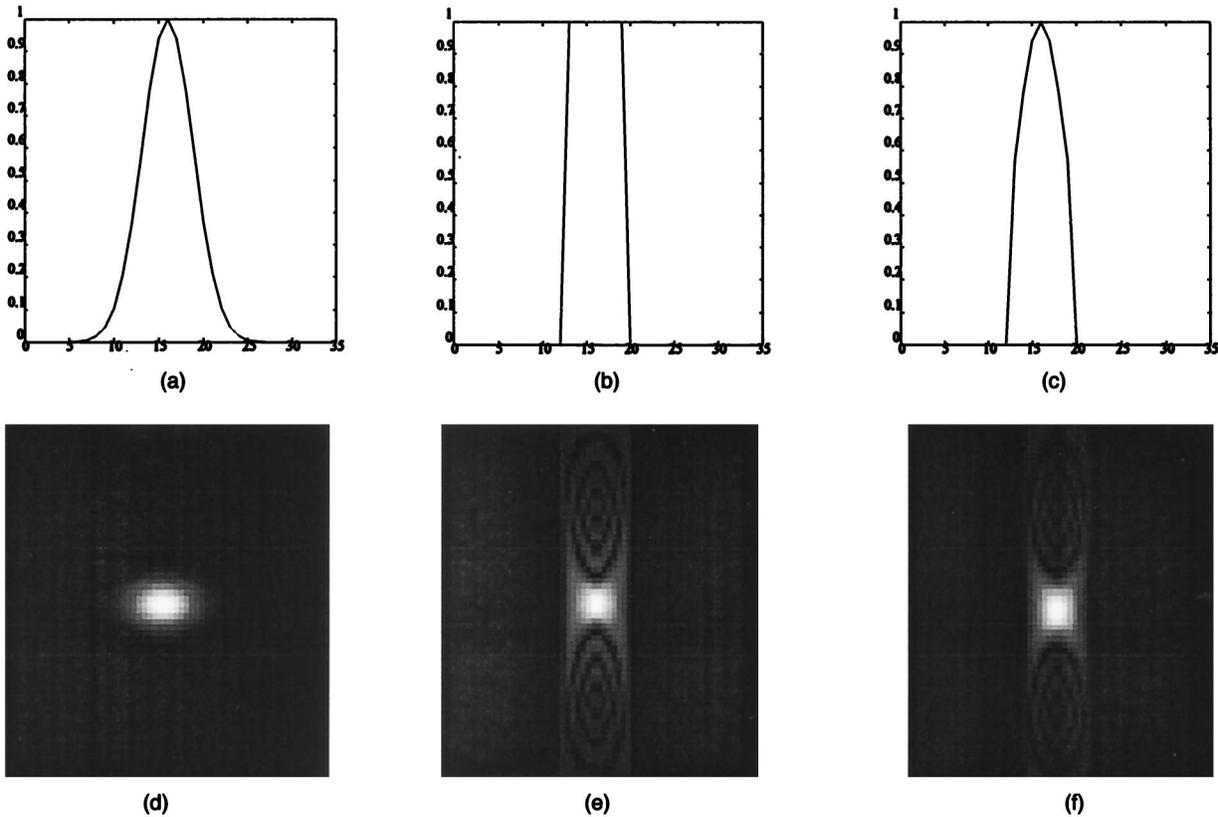
Fig. 5. Slitting of a Gaussian: (a) the Gaussian, (b) the slit, (c) the slitted Gaussian, (d)–(f) their corresponding Wigner functions.
