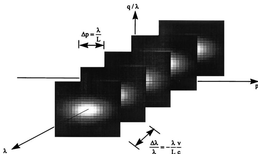
Fig. 4. Multiple copies of an originally monochromatic Wigner function separated by wavelength.
