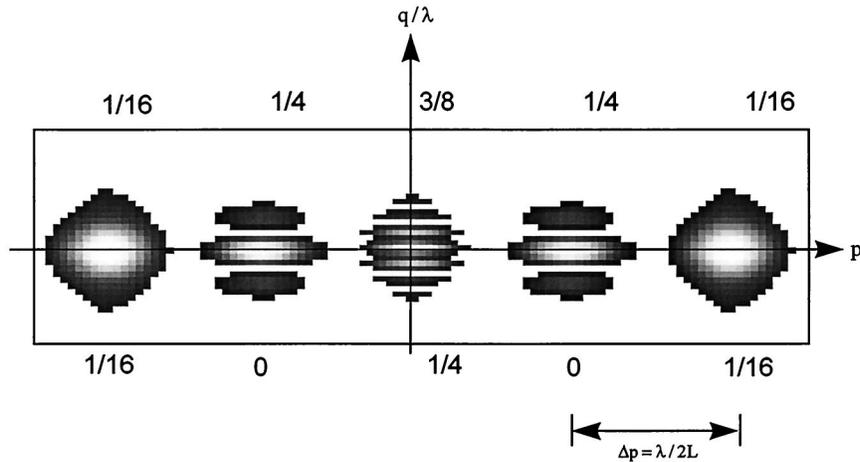
Fig. 3. Five replicas of a Wigner function produced by a cosinusoidal grating  $\Gamma^c(q) = 1/2[1 - \cos(2\pi q/L)]$  of period  $L$  in  $q$ . The replicas stand apart in the angle  $p \approx \theta$ . Above are the maxima of the coefficients  $W_n^r(q)$  of Eq. (4) (they sum to unity). Below are their rms values  $\langle W_n^r(q, t) \rangle$  of Eq. (9).
